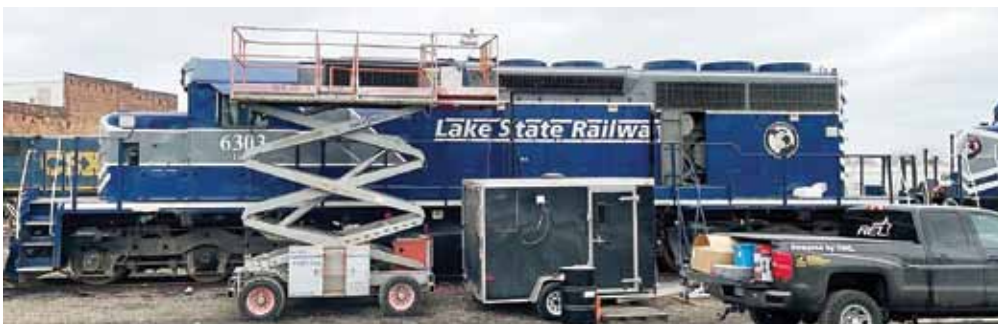
Emissions testing being conducted on a Lake State Railway locomotive. Photo courtesy of ASLRRA
