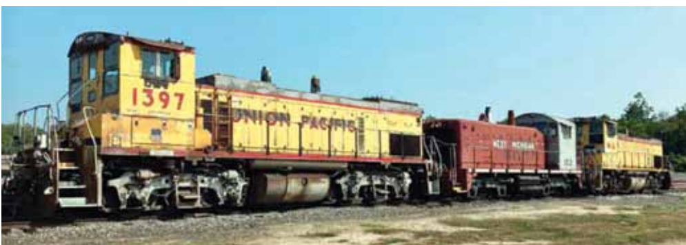
A trio of active locomotives await evening duty. Two former Milwaukee Road MP15AC's that wound up on UP sandwich an ex-GTW SW1200. Photo courtesy of Brian Buchanan/ Trains magazine.
